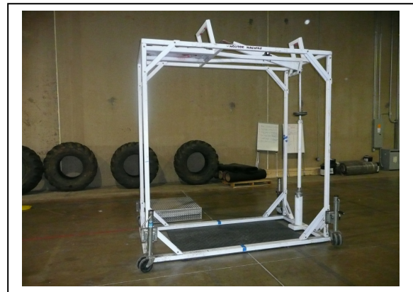
Hydraulic Ceiling Hook Test
